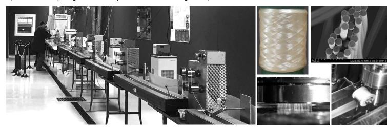
UKY CAER multifilament, continuous tow solution spinning line
